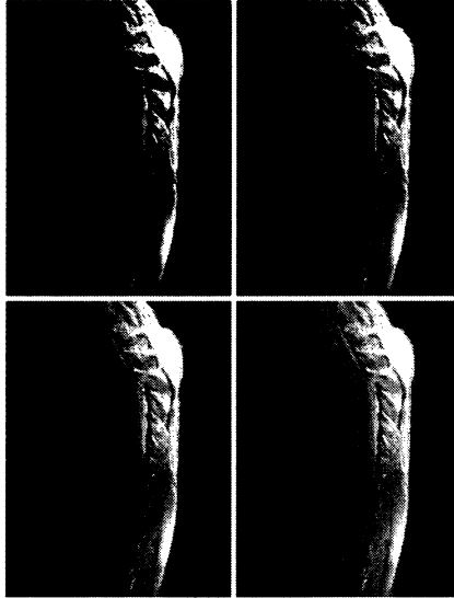
FIGURE 3.8 (a) Magnetic resonance (MR) image of a fractured human spine. (b)-(d) Results of applying the transformation in Eq. (3.2-3) with c = 1 and \gamma = 0.6, 0.4, and 0.3, respectively. (Original image for this example courtesy of Dr. David R. Pickens, Department of Radiological Sciences, Vanderbilt University Medical Center.)
