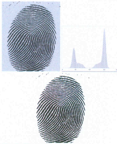
a b c FIGURE 10.29 (a) Original image. (b) Image histogram. (c) Result of segmentation with the threshold estimated by iteration. (Original courtesy of the National Institute of Standards and Technology.)
