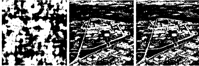
a b c FIGURE 5.28 Comparison of inverse- and Wiener filtering. (a) Result of full inverse filtering of Fig. 5.25(b). (b) Radially limited inverse filter result. (c) Wiener filter result.
