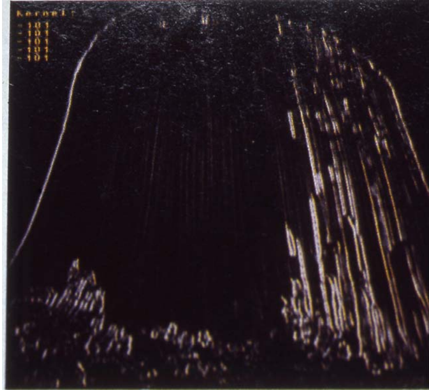
Photo 8: Convolution of photo 7 with a kernel (shown in the upper left corner) that amplifies vertical edges.
