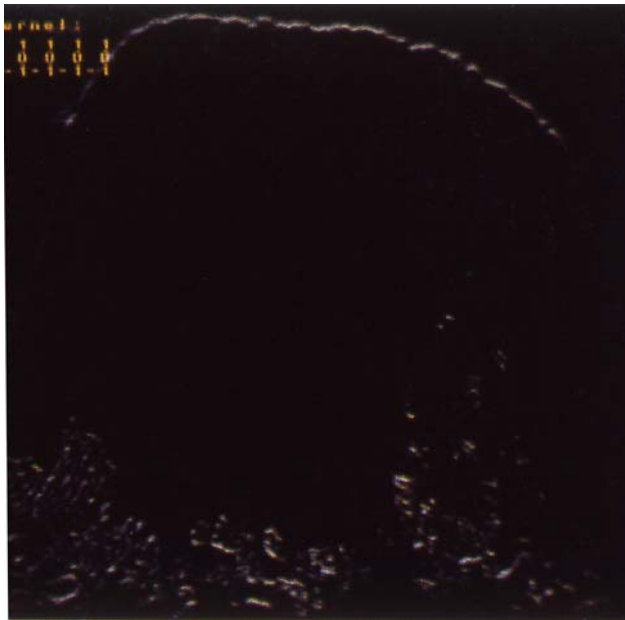
Photo 9: Convolution of photo 7 with kernel (shown in the upper left corner) that amplifies horizontal edges. As you can see, this image doesn't have many horizontal edges.
