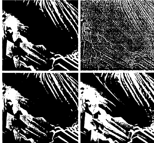
a b c d FIGURE 4.29 Same as Fig. 3.43, but using frequency domain filtering. (a) Input image. (b) Laplacian of (a). (c) Image obtained using Eq. (4.4-17) with A = 2 . (d) Same as (c), but with A = 2.7 . (Original image courtesy of Mr. Michael Shaffer, Department of Geological Sciences, University of Oregon, Eugene.)
