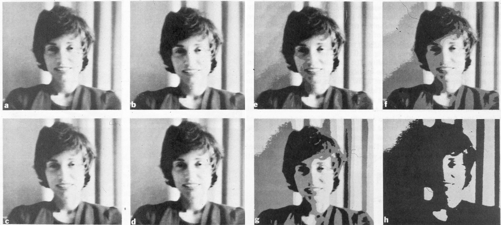
Figure 2.8. A 512 X 512 image displayed in 256, 128, 64, 32, 16, 8, 4, and 2 levels, respectively.
