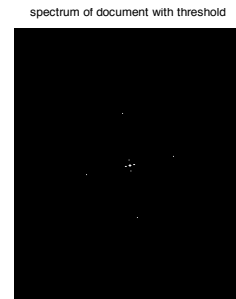
Figure 5 Binary image of the skew document in frequency domain
