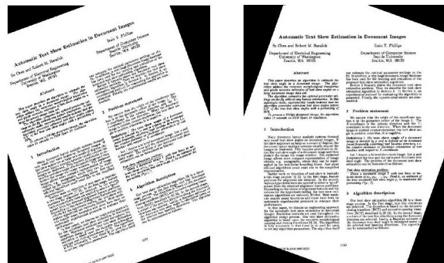
Figure 8.Original and skew corrected document image containing only text information
