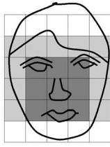
Fig. 2. A typical face used in knowledge-based top-down methods: Rules are coded based on human knowledge about the characteristics (e.g., intensity distribution and difference) of the facial regions [170].
