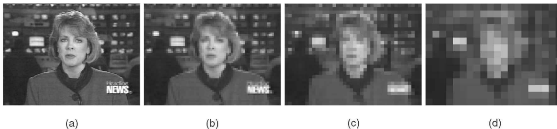
Fig. 1. (a) n = 1 , original image. (b) n = 4 . (c) n = 8 . (d) n = 16 . Original and corresponding low resolution images. Each square cell consists of n \times n pixels in which the intensity of each pixel is replaced by the average intensity of the pixels in that cell.
