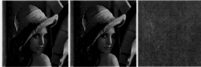
FIGURE 6.41 Image sharpening with the Laplacian. (a) Result of processing each RGB channel. (b) Result of processing the intensity component and converting to RGB. (c) Difference between the two results.
