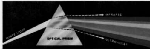
FIGURE 6.1 Color spectrum seen by passing white light through a prism. (Courtesy of the General Electric Co., Lamp Business Division.)
