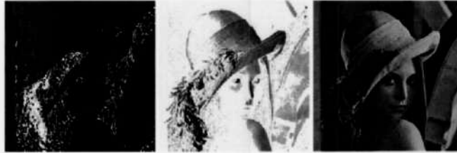
HSI components of the RGB color image in Fig. 6.38(a). (a) Hue. (b) Saturation. (c) Intensity.
