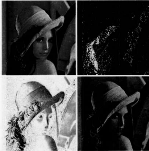
FIGURE 6.50 (a) RGB image with green plane corrupted by salt-and-pepper noise. (b) Hue component of HSI image. (c) Saturation component. (d) Intensity component.
