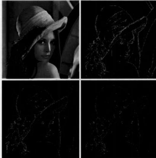
FIGURE 6.46 (a) RGB image. (b) Gradient computed in RGB color vector space. (c) Gradients computed on a per-image basis and then added. (d) Difference between (b) and (c).
