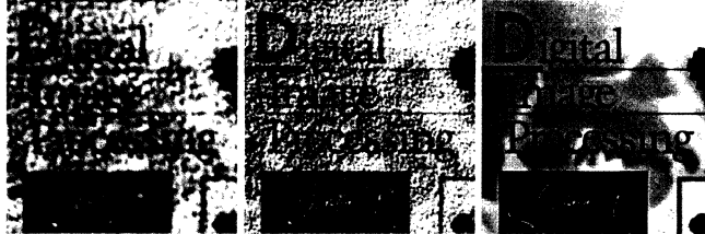
FIGURE 5.30 Results of constrained least squares filtering. Compare (a), (b), and (c) with the Wiener filtering results in Figs. 5.29(e), (f), and (i), respectively.
