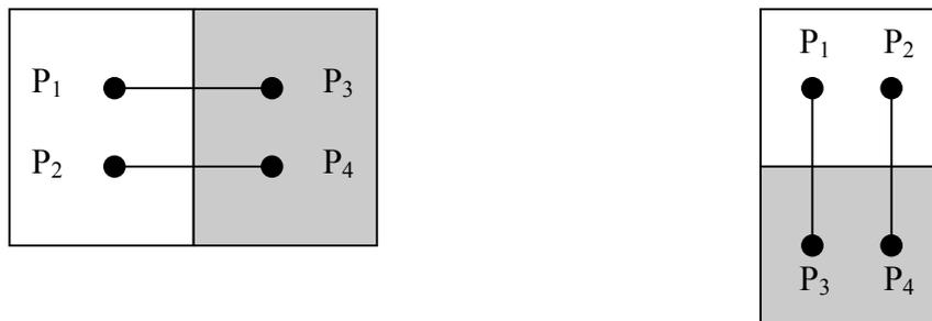
**Figure 7: 2 x 2 Prewitt method for edge detection**
