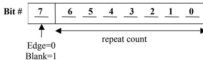
**Figure 10: Composition of compressed edge data byte**
