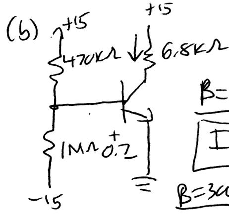
(b)  $I_B = \frac{15 - 0.7}{470k\Omega} - \frac{0.7 - (-15)}{1M\Omega} = 14.7 \mu A$
