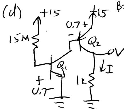
$$B=100 \quad I_{B1} = \frac{15 - 0.7}{15M} = 0.953 \mu\text{A} \quad I_{C1} = I_{B2} = 0.953 \mu\text{A}(100) = 95.3 \mu\text{A}$$
