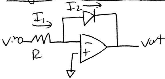
This circuit is connected just like a standard inverting amplifier, except that the feedback element is a diode, not a resistor. Since  $I_n = 0$ ,
