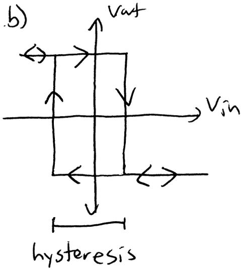
In this circuit, the hysteresis is the difference between the upper & lower trip points. The circuit will behave differently depending on the present output & the direction of the voltage change. This change in behavior is quantified as hysteresis, the range of  $V_{in}$  over which the circuit operation is different. Changing the trip voltages requires altering  $R_1$  &  $R_2$ .
