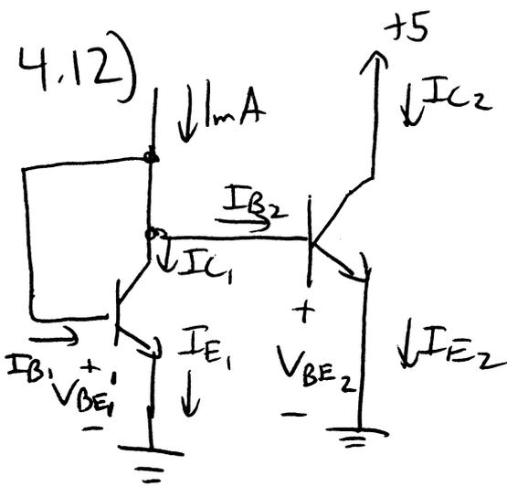
$$V_{BE1} = V_{BE2}, \quad \frac{I_{E1}}{I_{E2}} = \frac{I_{ES1}}{I_{ES2}} = 0.1 \therefore$$
