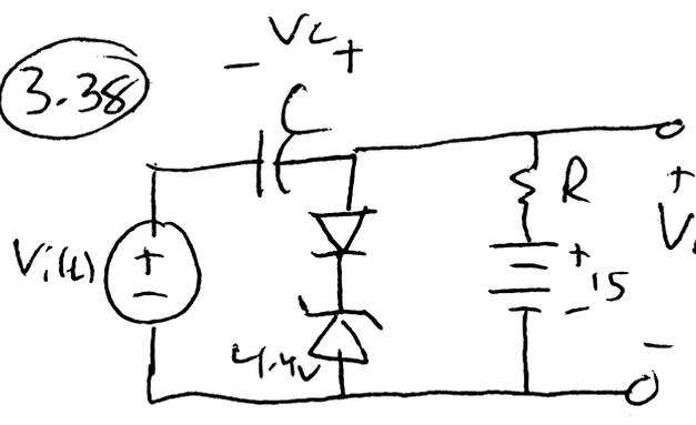
Circuit operation: With no input,  $V_i(t) = 0$ , Diodes will activate, charging capacitor until  $V_c = V_o = 5V$ . Then, diodes shut off. If
