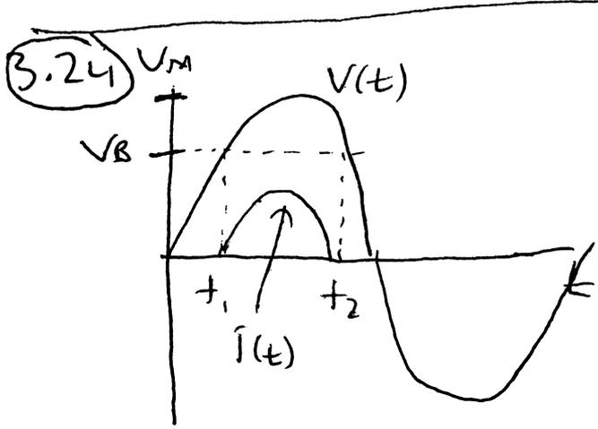
$i(t)$  is non-zero only when  $V(t) > V_B$ .  $i(t)$  will peak when  $V_s(t)$  peaks at  $V_m$ . Thus,  $i_{max} = \frac{V_m - V_B}{R}$   $i_{max} = 0.6 A$
