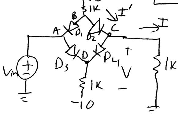
$V_{in} = 0 \rightarrow$  All diodes on.  $V_A = V_B = V_C = V_D = 0$ ,  $\boxed{V = 0, I = 0}$   $I' = 10mA$ , but all goes through  $D_4$  to -10.
