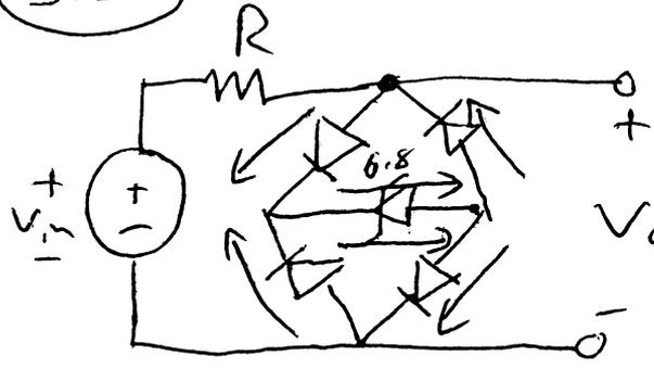
If the bridge is off,  $V_o = V_{in}$ . Once the bridge turns on,  $V_o$  will be held at that voltage. Higher voltages will cause more current over  $R$  & the output will be held at the initial "on" voltage.
