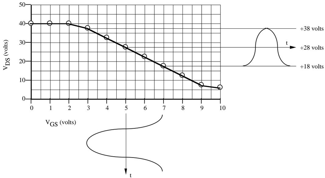
This circuit would make an excellent amplifier. It has a nice, long transfer curve and the input signal is approximately in the middle of the region resulting in undistorted output with a gain of approximately 5.
