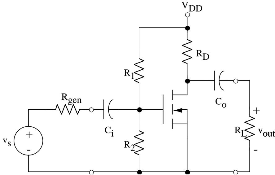
The circuit uses the values  $R_{gen}=10\text{k}\Omega$ ,  $V_{DD}=18\text{V}$ ,  $R_1=3.3\text{M}\Omega$ ,  $R_2=1.2\text{M}\Omega$ ,  $R_D=2\text{k}\Omega$ , and  $R_L=5\text{k}\Omega$ . The MOSFET is characterized by  $K=0.96\text{mA/V}^2$  and  $V_T=2.5\text{ volts}$ .
