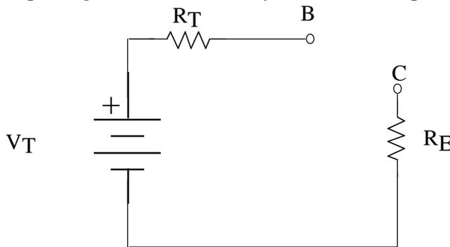
Doing KVL around this circuit we get  $-V_T + I_B R_T + V_{BE} + (\beta + 1)I_B R_E = 0$  which becomes  $-5.755 + I_B (3197\Omega) + 0.7 + (130 + 1)I_B (1000\Omega) = 0$  or  $I_B = \frac{5.055volts}{134197\Omega} = 37.67\mu A$ . Then  $I_{C,Q} = \beta I_B = (130)(37.67\mu A) = 4.897mA$ . Using this value we can compute  $V_{CE,Q}$  as
