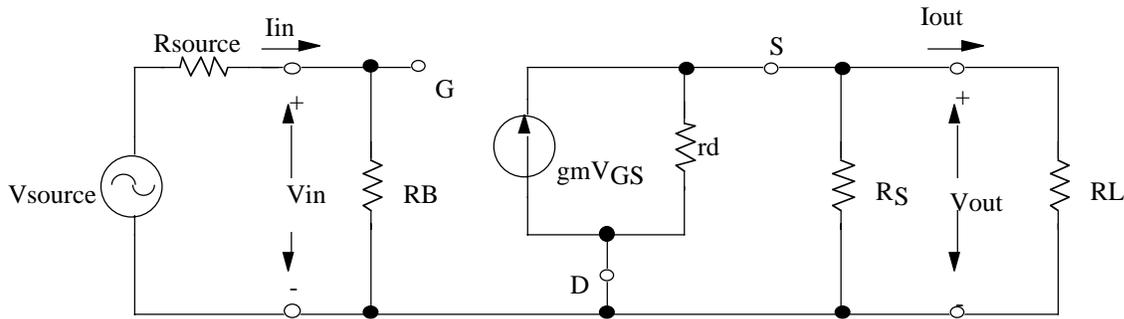
A student in EECS 245 has obtained the above small signal equivalent circuit for a MOSFET amplifier. The circuit parameters are  $R_{SOURCE}=100\Omega$ ,  $R_B=1.5M\Omega$ ,  $R_S=330\Omega$ , and  $R_L=100\Omega$ .
