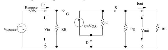
A student in EECS 245 has obtained the above small signal equivalent circuit for a MOSFET amplifier. The circuit parameters are  $R_{SOURCE}$ =100 $\Omega$ ,  $R_{B}$ =1.5 $M\Omega$ ,  $R_{S}$ =330 $\Omega$ , and  $R_{L}$ =100 $\Omega$ . The transistors small signal parameters are  $g_m$ =0.05S and  $r_d$ =100k $\Omega$ .
