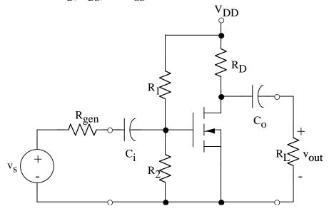
The circuit uses the values  $R_{gen}$ = 10k $\Omega$ ,  $V_{DD}$ =18V,  $R_1$ =3.3M $\Omega$ ,  $R_2$ =1.2M $\Omega$ ,  $R_D$ =2k $\Omega$ , and  $R_L$ =5k $\Omega$  The MOSFET is characterized by K=0.96mA/V<sup>2</sup> and  $V_T$ =2.5 volts.
