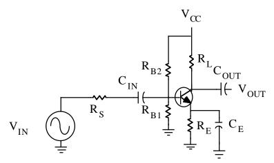
Consider the above BJT amplifier where  $R_S=500\Omega$ ,  $R_{B1}=2.7k\Omega$ ,  $R_{B2}=7.5k\Omega$ ,  $R_E=200\Omega$ ,
