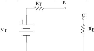
Doing KVL around this circuit we get  $-V_T + I_B R_T + V_{BE} + (\beta + 1)I_B R_E = 0$  which becomes  $-5.755 + I_{\scriptscriptstyle B}\big(3197\Omega\big) + 0.7 + \big(130+1\big)I_{\scriptscriptstyle B}\big(1000\Omega\big) = 0 \text{ or } I_{\scriptscriptstyle B} = \frac{5.055 volts}{134197\Omega} = 37.67 \mu A \,. \text{ Then } I_{\scriptscriptstyle B} = 1.000 \,.$  $I_{C,Q} = \beta I_B = (130)(36.67 \mu A) = 4.897 mA$ . Using this value we can compute  $V_{CE,Q}$  as
