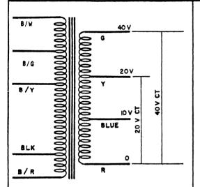
These transformers are designed for use with silicon diode rectifiers, to supply the DC voltages for transistors in their various applications. They are intended for use with full wave bridge or bridge rectifier, but may be used with voltage doubler circuits at one-half of the rated current.
