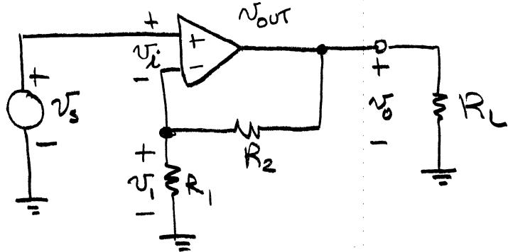
positive output to inverting input  $\rightarrow$  NEGATIVE feedback
