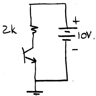
$$V_{OC} = 10 \text{ volts.}$$
