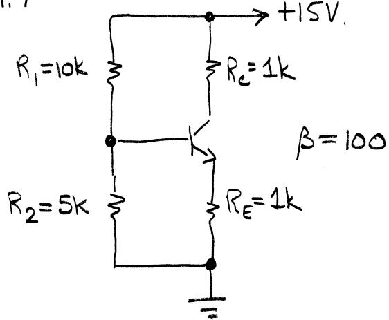
Thevenize the input:  $V_{BB} = \frac{5k}{5k+10k} \cdot 15V = \frac{5}{15} \cdot 15 = 5$  volts.
