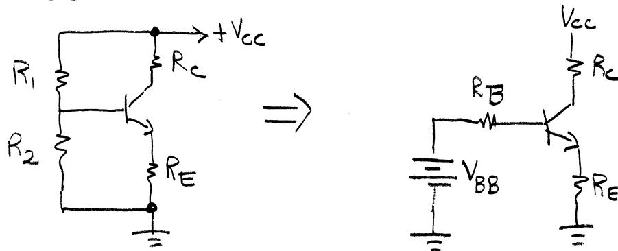
where  $R_B, V_{BB}$  are the Thevenin equivalent of the bias circuit
