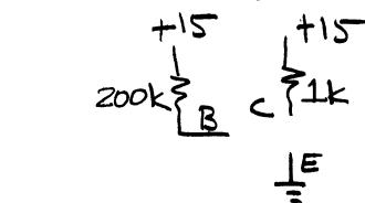
$$I_c = \frac{V_{cc} - 0.2}{1k} = \frac{15 - 0.2}{1k} = 14.8 \text{ mA}$$
