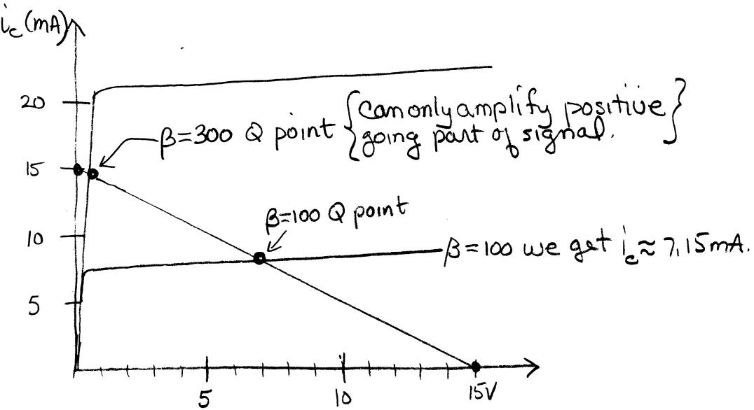
load line  $V_{ce} = 15 V$
