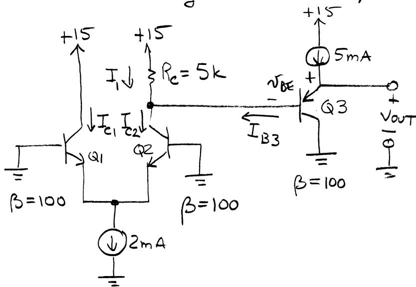
Since  $Q_1, Q_2$  are identical and their  $V_{BE}$ 's are identical
