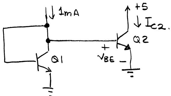
Shockley equation  $i_E = I_{ES} \left[ e^{\frac{V_{BE}}{V_T}} - 1 \right]$
