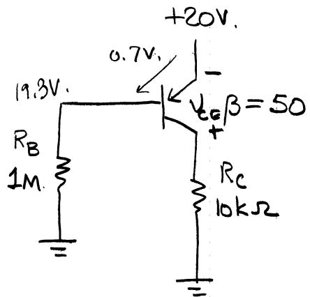
(a) transistor is not cutoff since  $V_{BE} > 0.5$  volts.
