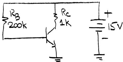
$$I_B = \frac{V_{cc} - 0.7}{R_B} = \frac{15 - 0.7}{200k} = 71.5 \mu A.$$
