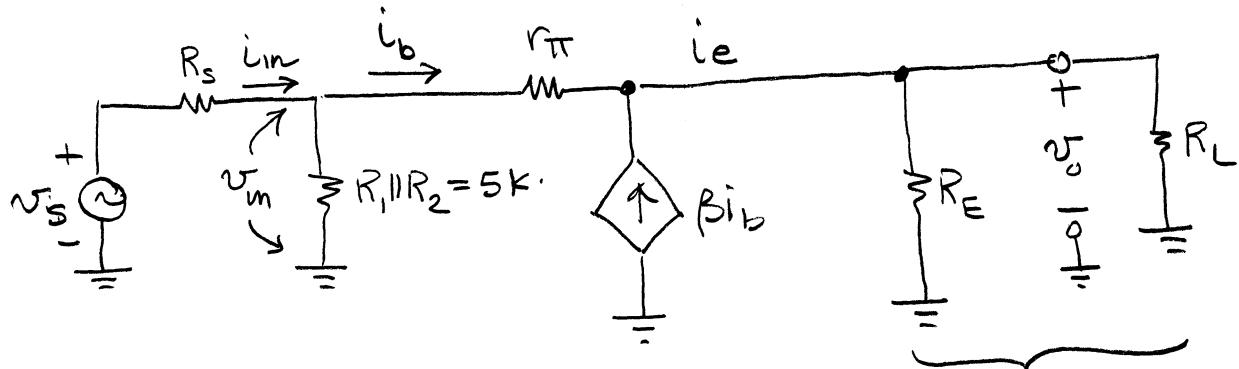
$$R'_L = R_E \parallel R_L = \frac{(1000)(500)}{1000 + 500} = 333 \Omega$$
