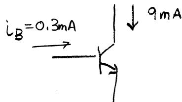
$$i_E = i_C + i_B = 9\text{mA} + 0.3\text{mA} = 9.3\text{mA}$$
