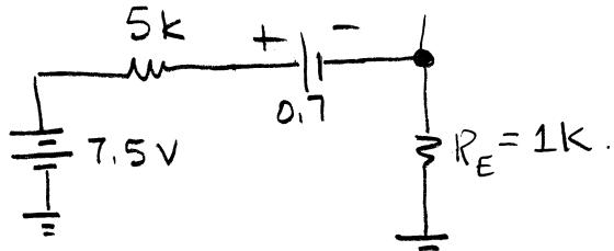
$$\text{doing KCL} \quad -7.5 + i_B(5k) + 0.7 + (\beta i_B)(1k) = 0$$
