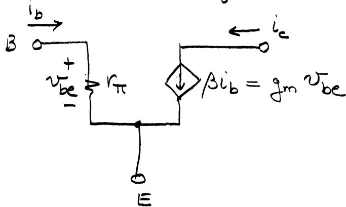
4.42 (partial) An npn silicon transistor at room temperature has  $\beta=100$ .
