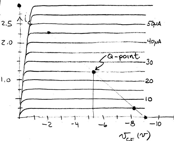
load line  $V_{oc} = -0.8$  Volts.
