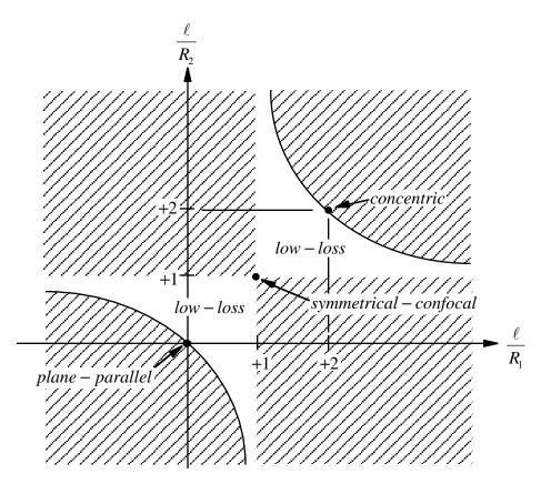
Stability diagram of an optical resonator
