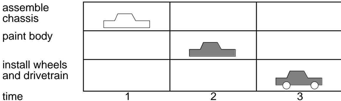
A conventional process would require 9 time units to produce three cars.
