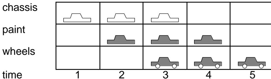
A pipelined process would require 5 time units to produce the same number of cars.
