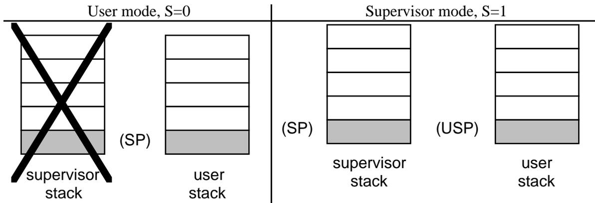
Bit 13 of the status register is used to toggle A7 between the user and supervisor modes. USP references the user stack while the 68000 is in supervisor mode.
