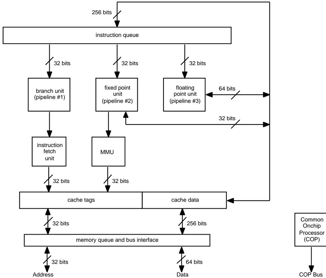
NOTE: The COP processor controls built-in self test, debug and test features at boot time.
