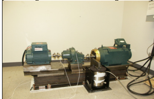
Motor and Gearbox Vibration Test Rig • Rotor Faults • Stator Winding Faults • Motor Bearing Faults • Gear Bearing Faults • Gear Faults
