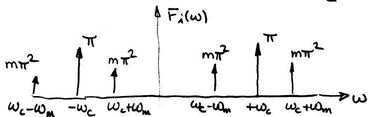
$F_o(\omega)$  will consist of these impulses multiplied by the wave impedance at that frequency  $\left[ 120\pi w \left( \omega^2 - \frac{c^2\pi^2}{6.25} \right) \right]$
