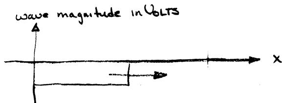
a wave of  $-V_0$  volts traveling in the  $+x$  direction
