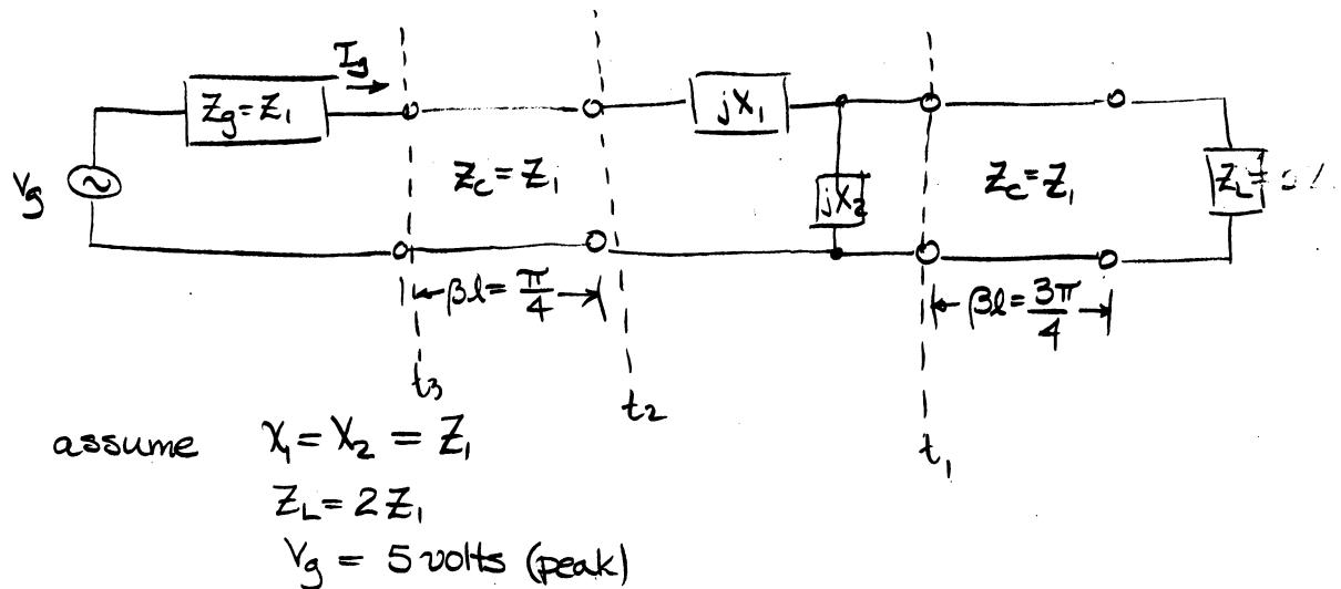
transform  $Z_L$  to plane  $t_3$  using intermediate planes  $t_1$  and  $t_2$
