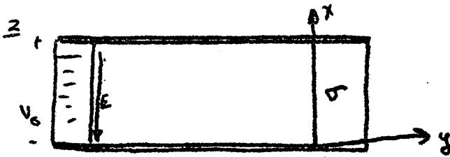
a. If the top and bottom plates have infinite conductivity then there can be no tangential  $E$  on their surfaces.
