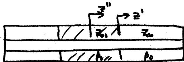
the impedance of a coaxial cable,  $Z_0 = \sqrt{\frac{\mu}{\epsilon}} \frac{\ln \frac{b}{a}}{2\pi}$
