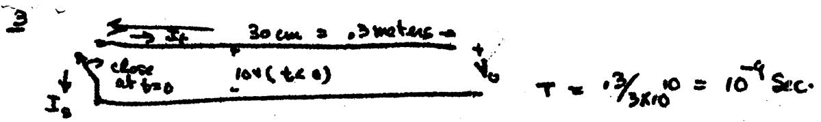
at  $t=0$  switch closes and  $I_+ = -\frac{10}{Z_0} = -10 \text{ amps}$
