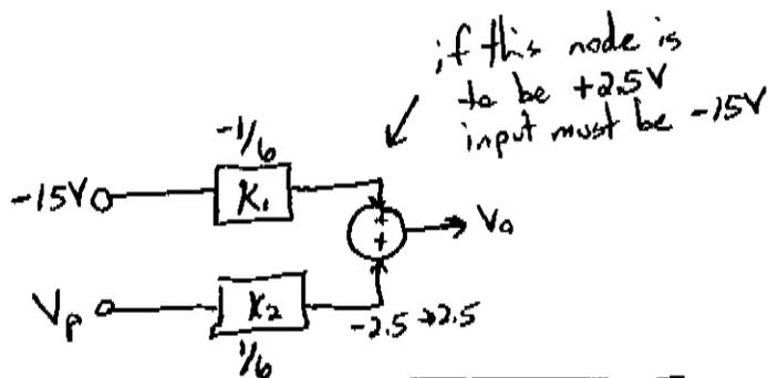
$$\frac{R_2}{R_1} = \frac{1}{6} \quad \frac{R_4}{R_3} = \frac{1}{6}$$
