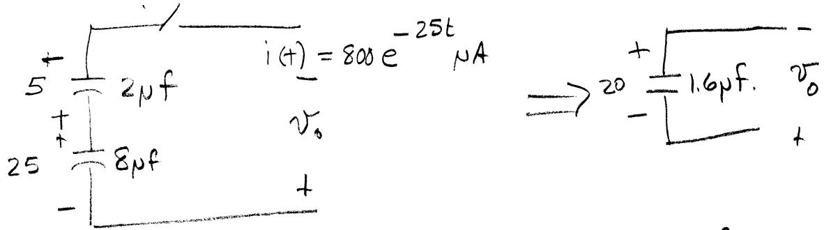
$$(a) \frac{1}{C_{EQ}} = \frac{1}{2} + \frac{1}{8} = \frac{4}{8} + \frac{1}{8} = \frac{5}{8} \quad C_{EQ} = \frac{8}{5} = 1.6 \mu F.$$
