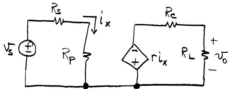
$$\text{For the input circuit} \quad i_x = \frac{v_s}{R_s + R_p}$$
