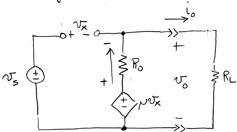
$$\text{Do KVL across input} \quad -v_s + v_x + v_o = 0 \Rightarrow v_x = v_s - v_o$$
