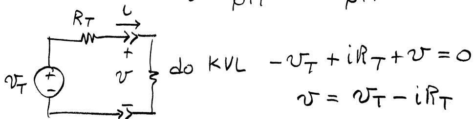
$$\Rightarrow v_T = \frac{\mu}{\mu + 1} v_s \quad R_T = \frac{R_o}{\mu + 1}$$
