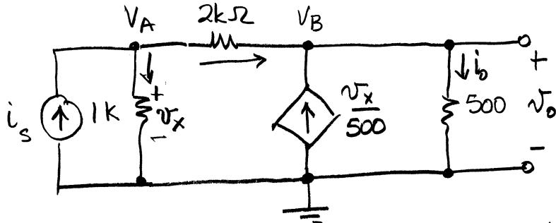
$$\text{KCL at } A: \sum_i = 0 \quad +i_s - \frac{V_A - 0}{1k} - \frac{V_A - V_B}{2k} = 0$$
