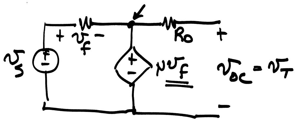
$$\text{do KVL at input} \quad -V_s + V_f + N V_f = 0$$
