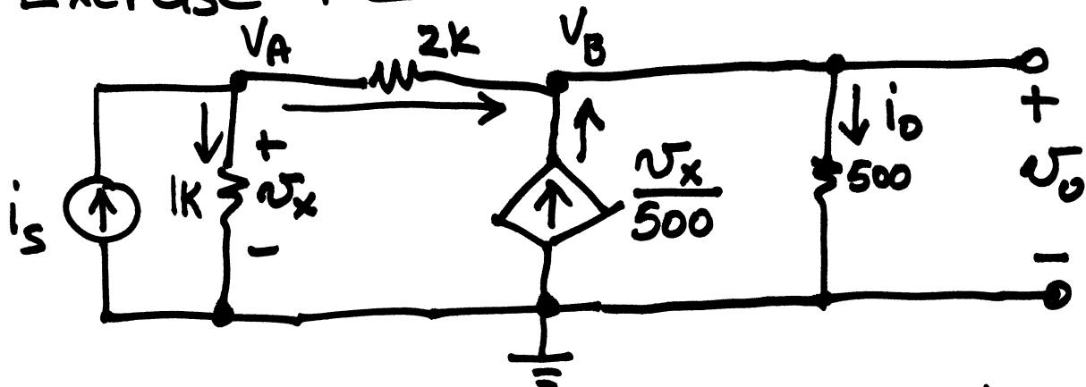
$$\text{KCL @ A} \quad \sum_{\text{in}} i = 0 \quad +i_s - \frac{v_A - 0}{1K} - \frac{v_A - v_B}{2K} = 0$$
