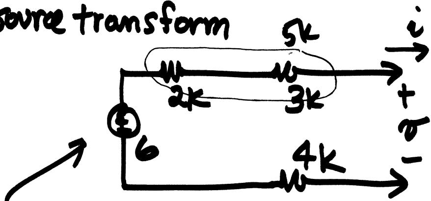
$$U = iR = \left(3 \text{mA}\right) \left(2 \text{k}\right) = 6 \text{volts}$$
