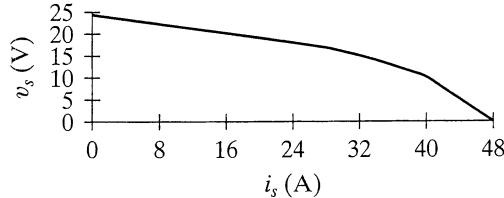
b) 24 V source;  $0.25 \Omega$  resistor
