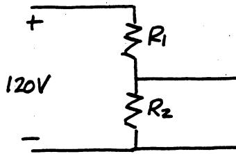
Maximum dissipation in  $R_2$  occurs at no load,  $\therefore$
