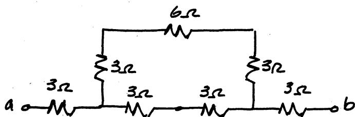
Now the  $12\Omega$  in parallel with  $6\Omega$  reduces to  $R_2 = \frac{(12)(6)}{18} = 4\Omega$
