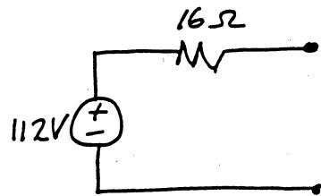
**P 4.56** After replacing the  $40\Omega$ - $10\Omega$ - $8\Omega$  wye with an equivalent delta the circuit becomes
