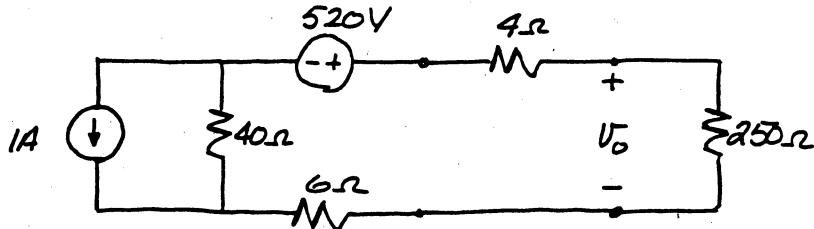
Next use a source transformation to convert the 1-A current source and  $40\Omega$  resistor
