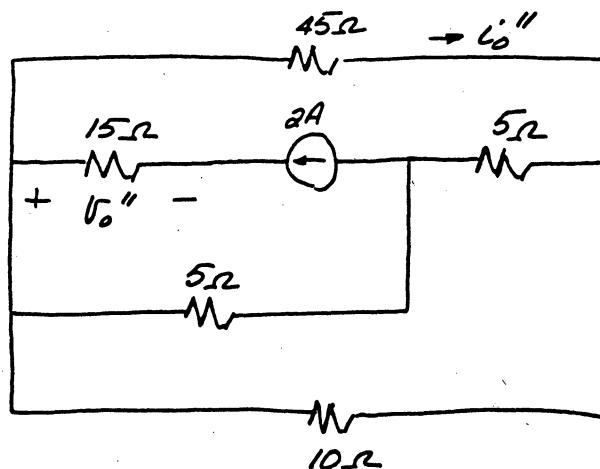
The  $15\Omega$  resistor will have no effect on  $i_o''$  since it is in series with a 2-A source.
