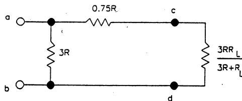
$$\text{Now note: } 0.75R + \frac{3RR_L}{3R + R_L} = \frac{2.25R_L^2 + 3.75RR_L}{3R + R_L}$$
