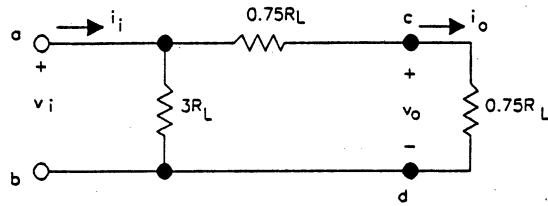
$$i_o = \frac{i(3R_L)}{4.5R_L} = \frac{1}{1.5}i = \frac{1}{1.5} \frac{v_i}{R_L}, \quad v_o = 0.75R_L i_o = \frac{1}{2}v_i,$$
