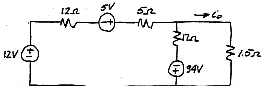
Now combine the 12-V and 5-V sources into a single voltage source and the 12-Ω and 5-Ω resistors into a single resistor, to get
