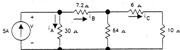
$$16//64 = 12.8 \Omega, \quad 12.8 + 7.2 = 20 \Omega, \quad 20//30 = 12 \Omega$$
