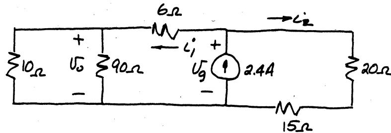
$10//90 = 9 \Omega, \quad 9 + 6 = 15 \Omega, \quad 15 + 20 = 35 \Omega$
