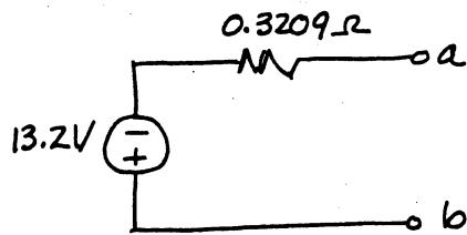
[b] The output resistance of the inverting amplifier is the same as the Thévenin resistance, i.e.,
