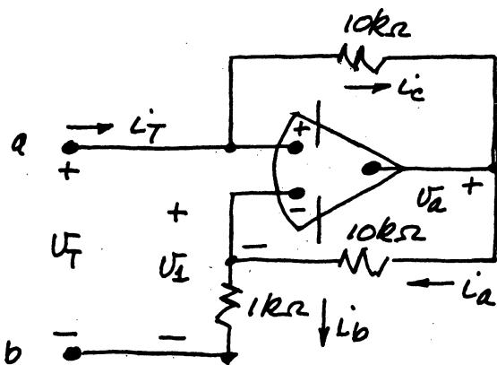
Apply a test voltage across a, b and note
