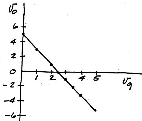
[ b ] Yes, the output voltage is bipolar, i.e.,  $-5 \text{ V} \leq v_o \leq 5 \text{ V}$  and the input voltage is unipolar  $0 \leq v_g \leq 5 \text{ V}$ .
