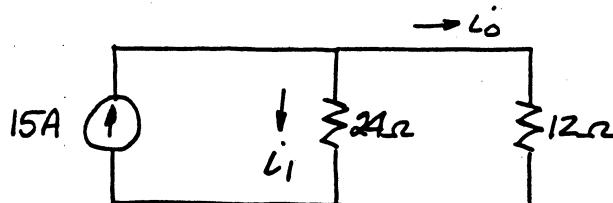
$$i_o = \frac{(15)(24)}{(24 + 12)} = \frac{2}{3}(15) = 10\text{ A}; \quad P_{12\Omega} = (10)^2(12) = 1200\text{ W}$$
