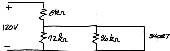
$$P_{R_1} = \frac{(120)^2}{8000} = 1.8 \text{ W} = 1800 \text{ mW}$$
