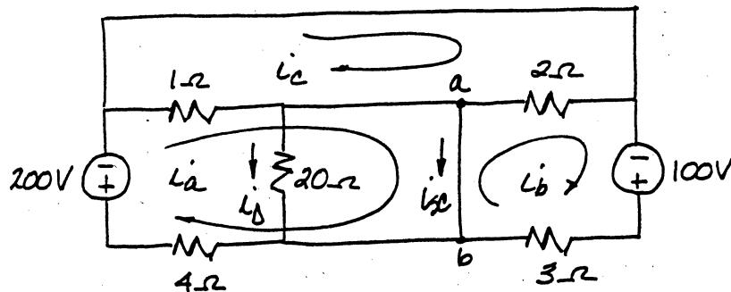
Note with the short circuit from a to b that  $i_\Delta$  is zero, hence  $14i_\Delta$  is also zero.
