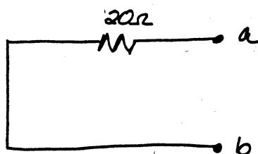
**P 4.67**  $V_{Th} = 0$ , since circuit contains no independent sources.
