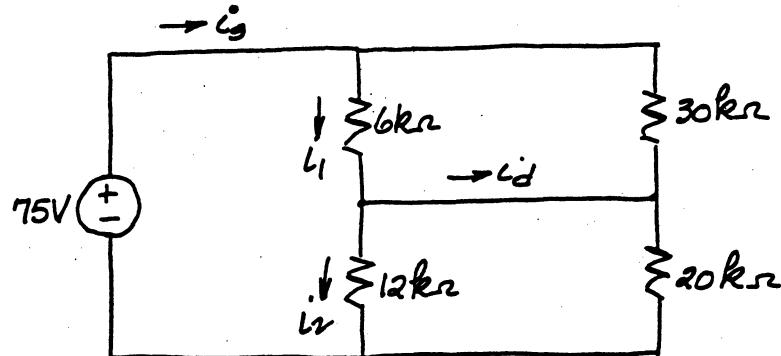
$$6 \text{ k}\Omega // 30 \text{ k}\Omega = 5 \text{ k}\Omega$$
