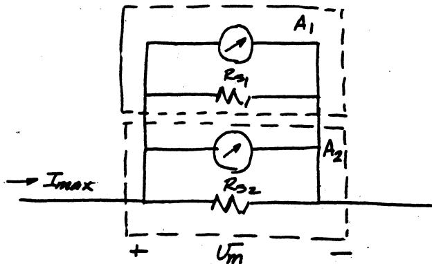
Note the maximum voltage across the parallel-connected ammeters is limited to  $500 \mu\text{V}$ , otherwise ammeter 1 exceeds its full-scale reading.
