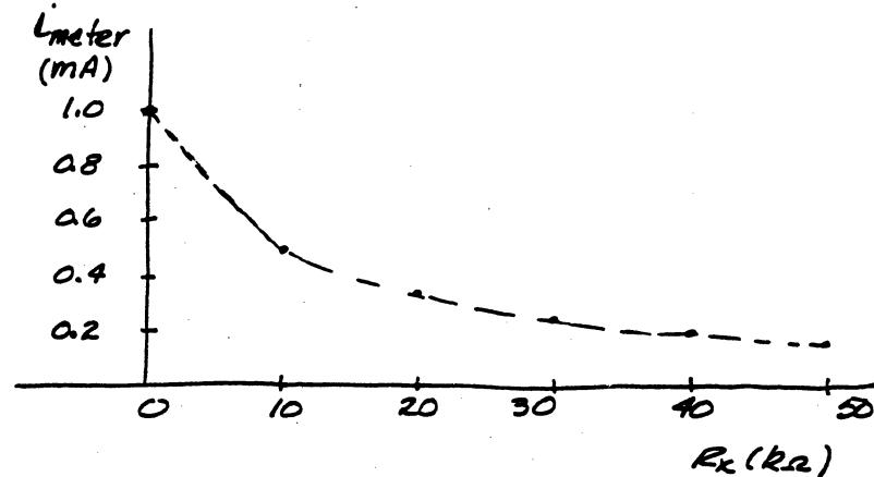
[c] Because the meter current varies nonlinearly with respect to  $R_x$  but the deflection of the meter is proportional to  $i_{\text{meter}}$ .
