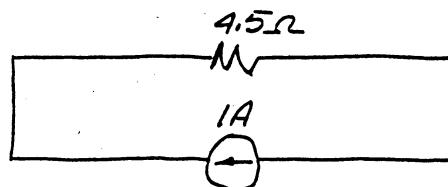
Therefore the voltage across the  $45\text{-}\Omega$  resistor is  $4.5\text{ V}$ , hence  $i_o'' = \frac{4.5}{45} = 0.10\text{ A}$
