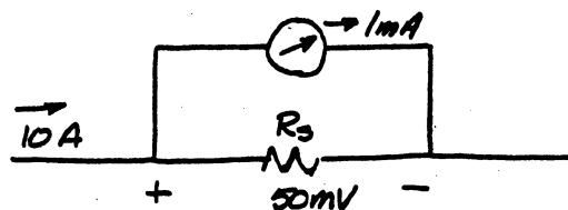
$$\text{Original meter: } R_e = \frac{50 \times 10^{-3}}{10} = 5 \times 10^{-3} = 0.005 \Omega$$
