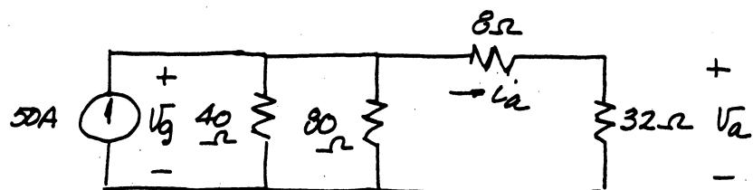
Now  $40\Omega \parallel 80\Omega \parallel 40\Omega = 16\Omega$ .
