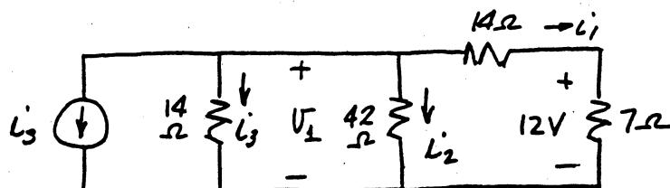
$$i_1 = \frac{12}{7}\text{ A}; \quad v_1 = (21)\left(\frac{12}{7}\right) = 36\text{ V}$$
