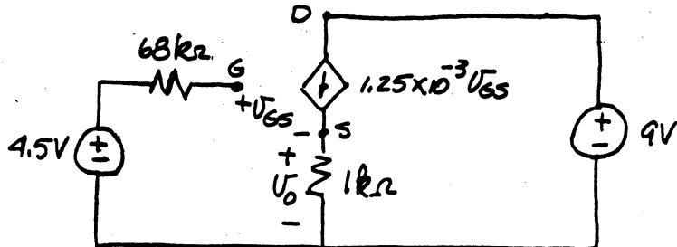
$$4.5 = v_{GS} + 1000(1.25 \times 10^{-3} v_{GS}) = 2.25 v_{GS}, \quad \therefore v_{GS} = \frac{4.5}{2.25} = 2 \text{ V}$$
