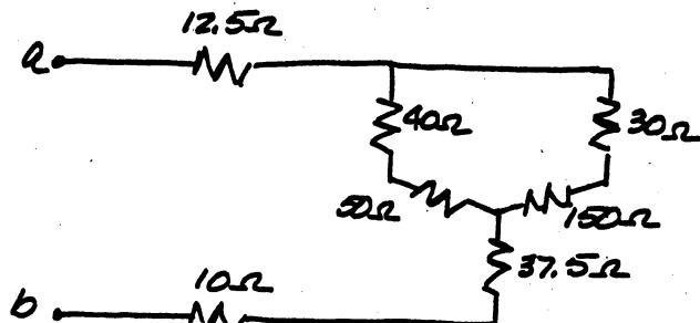
$$50\Omega + 40\Omega = 90\Omega, \quad 150\Omega + 30\Omega = 180\Omega$$
