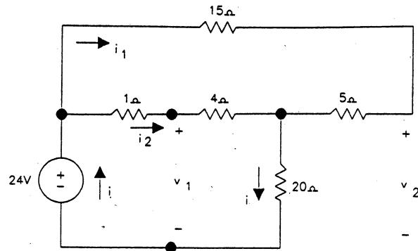
$$[b] \quad i_1 = (5/25)i = 0.2 \text{ A}, \quad i_2 = 1 - 0.2 = 0.8 \text{ A}$$
