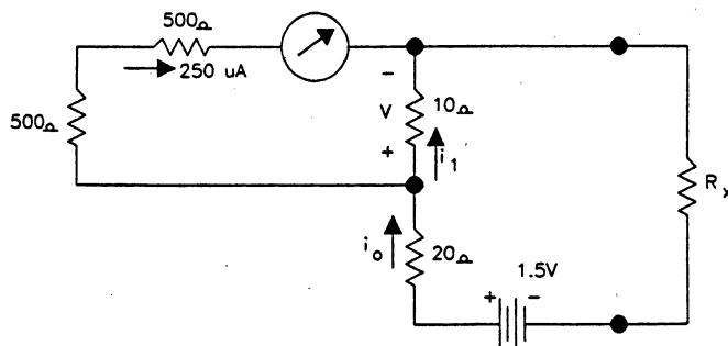
$$v = 1000(250) \times 10^{-6} = 0.25 \text{ V}, \quad i_1 = 0.25/10 = 25,000 \mu\text{A},$$
