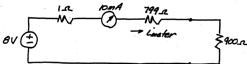
$$i_{\text{meter}} = \frac{8}{800 + 900} = \frac{8}{1700} \text{ A}$$
