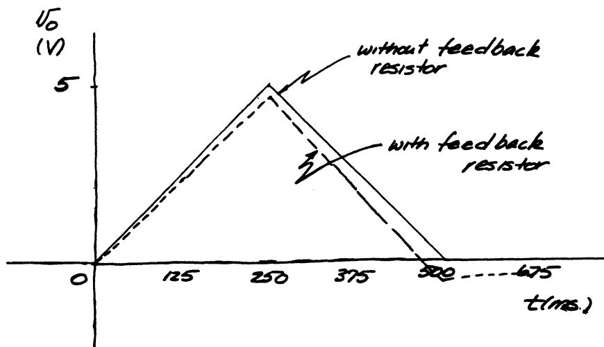
**P 8.84 [a]**  $R_f C_f = (400 \times 10^3)(0.05 \times 10^{-6}) = 20 \text{ ms}; \quad \frac{1}{R_f C_f} = 50; \quad \frac{R_f}{R_s} = 12.5$
