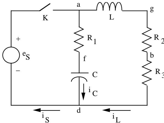
You are given that  $e_S(t) = E + E_1 \sin(500t) + E_2 \sin(1000t)$ ,  $L = 10$  millihenries,  $C = 200$  microfarads,  $R_1 = 10$  ohms,  $R_2 = 5.0$  ohms and  $R_3 = 5.0$  ohms in the above circuit.
