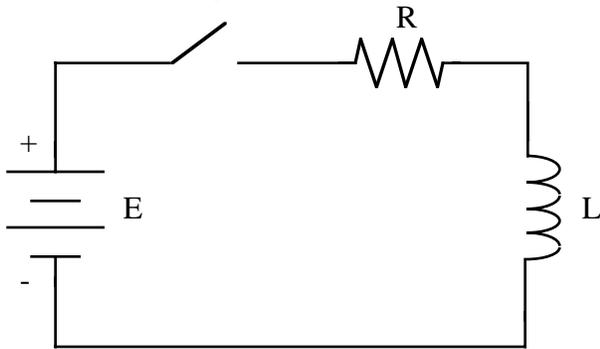
The question is what is the current in the circuit as a function of time for  $t \geq 0$ , the switch closes at  $t=0$ . This requires the use of differential equations. To describe this circuit begin with Kirchoff's voltage law
