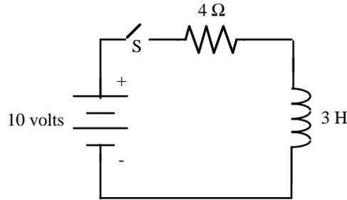
We use KVL to write the differential equation for the circuit using the correct expression for the impedance of the inductor.
