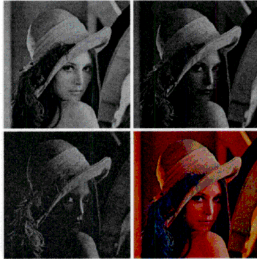
FIGURE 6.48 (a)–(c) Red, green, and blue component images corrupted by additive Gaussian noise of mean 0 and variance 800. (d) Resulting RGB image. [Compare (d) with Fig. 6.46(a).]
