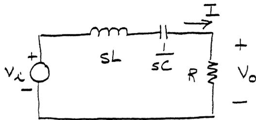
$$I(s) = \frac{V_i(s)}{sL + \frac{1}{sC} + R} = \frac{V_i(s) \left(\frac{s}{L}\right)}{s^2 + \frac{R}{L}s + \frac{1}{LC}}$$
