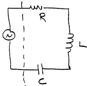
$$Z_{in}(j\omega) = R + j\omega L + \frac{1}{j\omega C} = R + j\left(\omega L - \frac{1}{\omega C}\right)$$
