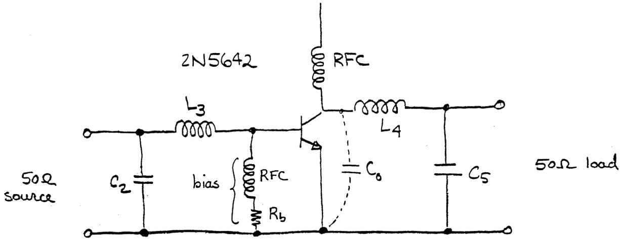
from data sheet for transistor  $Z_o @ 175\text{MHz} = 12.2 - j13.55$  (capacitive)
