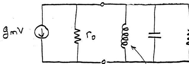
$$Q_p = \frac{R_p}{\omega_0 L} \rightarrow \frac{R_p}{\omega_0 \frac{1}{\omega_0^2 C}} = \omega_0 R_p C$$
