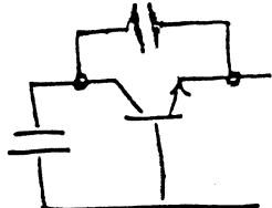
This circuit is a capacitive feedback oscillator. If  $\text{Re}(y_{\text{out}}) < 0$  it will oscillate.
