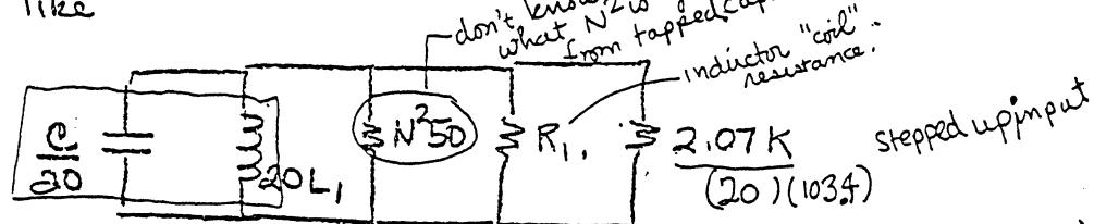
Note that because the coil inductance increased by 20, the capacitance must decrease by 20 to maintain the same resonant frequency. The Q of this circuit is determined by the resistors, since,
