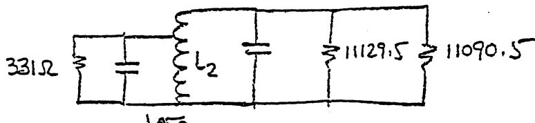
The current value of  $L_2$  is determined by the tank circuit to the right of the transformer (this is chosen for convenience) since  $R_2$  (the coil resistance) is defined there.
