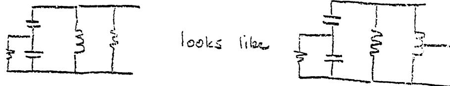
If we choose a transformer with a 20:1 impedance ratio we find the input impedance of  $103.4 \Omega$  stepped up to get  $2.07 \text{ k}\Omega$ . The resulting circuit looks like
