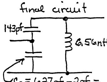
$$C_2 = 627 \text{ pF} - 2 \text{ pF} = 625 \text{ pF}$$
