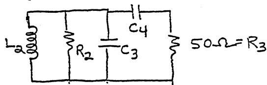
where  $R_2$  is the parallel equivalent resistance of the inductor.
