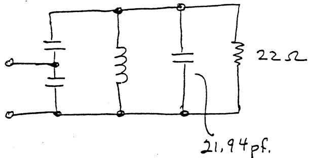
It is impossible to match any resistance greater than  $22\Omega$  using this network.
