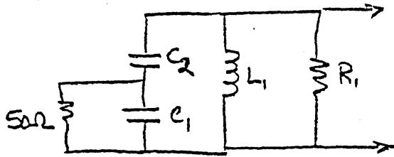
where  $R_1$  is the <sup>(parallel)</sup> resistance of  $L_1$
