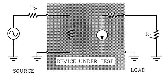
There is, as we know from our discussion on noise, a maximum of power transferred from one circuit to another when they are conjugately matched. To illustrate this point, we introduce the fictitious concept of Matching Factor (or MF). The MF is simply the ratio of the actual power transferred from one device to another to the available power from the source. For the circuit shown below this may be simply calculated.
