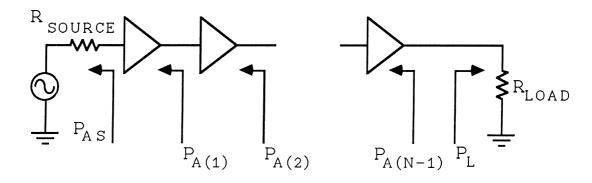
$$A_{T} = \frac{P_{L}}{P_{AS}} = \frac{P_{A1}}{P_{AS}} \times \frac{P_{A2}}{P_{A1}} \times \dots \times \frac{P_{An}}{P_{A(n-1)}} \times \frac{P_{L}}{P_{An}}$$
