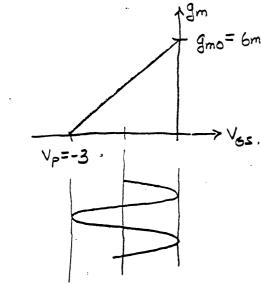
$$g_c = \frac{I_{IF}}{V_{RF}} = \frac{g_{ma} V_{Lo}}{2|V_{p}|}$$
