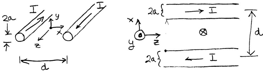
Superimpose the field from each conductor modeling the fields as those from two infinitely long parallel lines.
