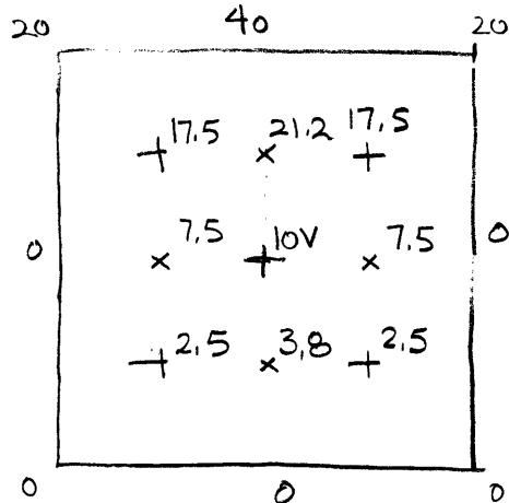
Now find the potential for each of the four sub-boxes. Assume the voltage at the trough-lid gap is the average (i.e.  $\frac{40+0}{2} = 20$ )
