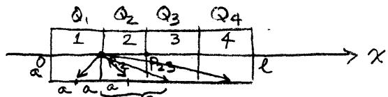
Let the total charge on segment 1 be  $Q_1$ ; the charge on segment 2 be  $Q_2$ . By symmetry  $Q_3 = Q_2$  and  $Q_4 = Q_1$ .
