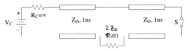
Assume the switch S is closed at S=0. Sketch the behavior of the voltage  $\mathcal{V}_0$  as a function of time.
