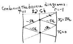
The following explains how the Blumlein configuration for transmission lines achieves the charge voltage into a matched load for a pulse length equal in length to the double transit time of one of two lines.
