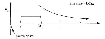
The following explains how the Blumlein configuration for transmission lines achieves the charge voltage into a matched load for a pulse length equal in length to the double transit time of one of two lines.
