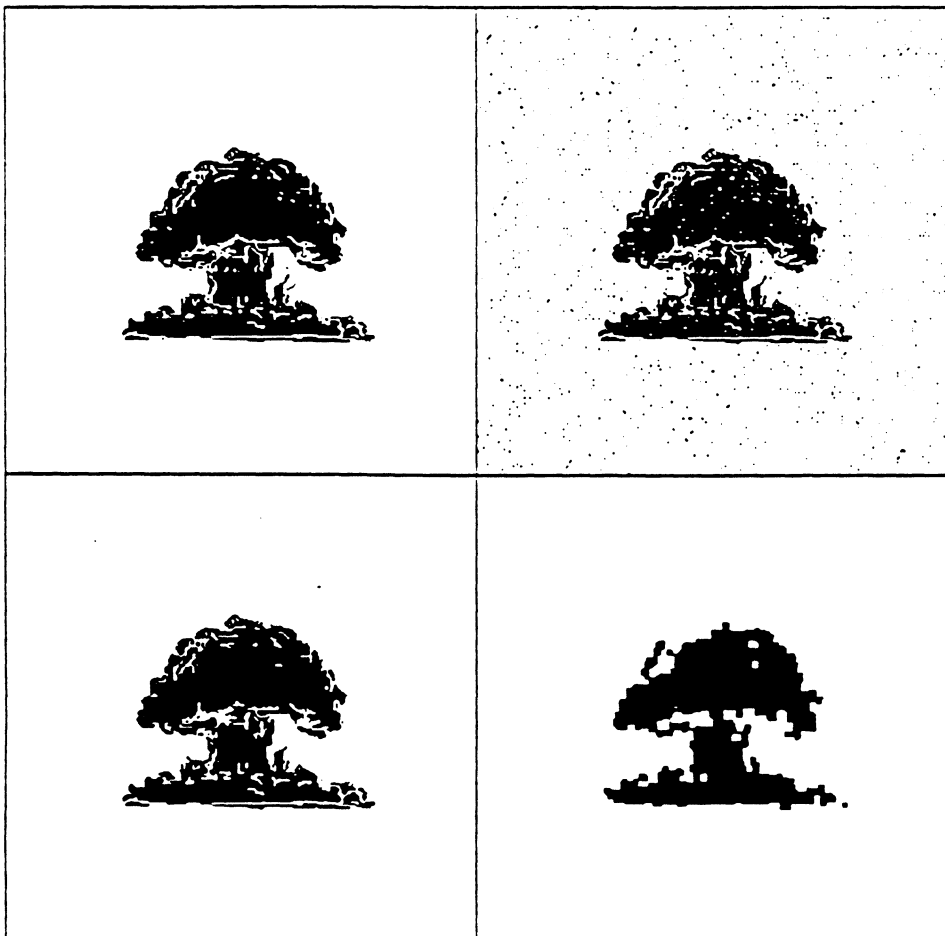
FIG. 9. Upper left: original image; upper right: noisy version of the original image; lower left: resultant image from a complex binary morphological filter using the eight structuring elements
