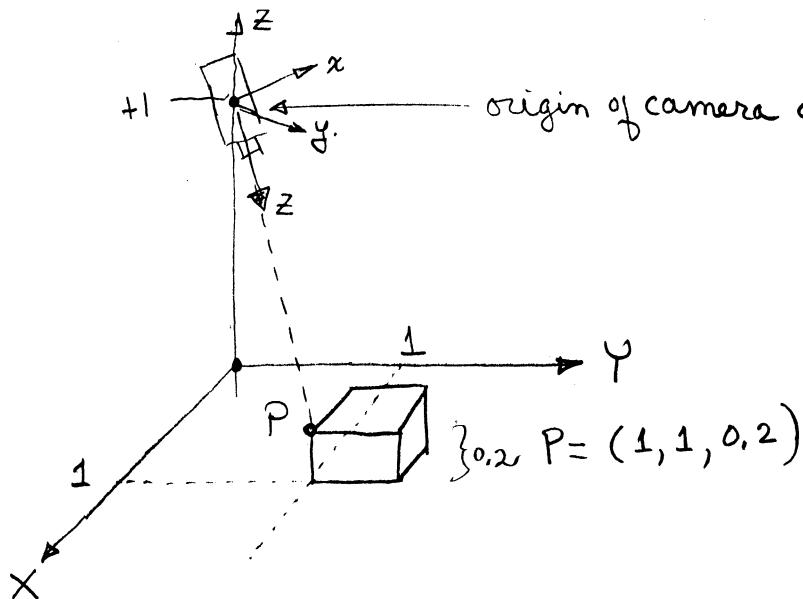
The camera is viewing point P. The camera is offset from the origin of the  $(x, y, z)$  coordinate system and has a pan =  $45^\circ$ , tilt =  $135^\circ$ .
