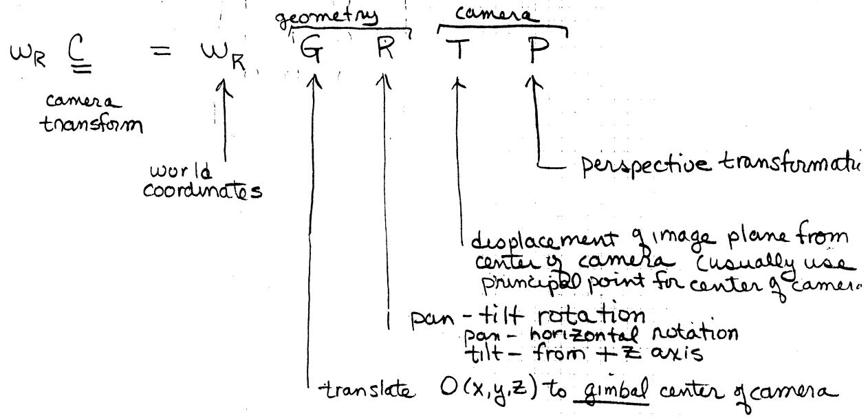
In general, we can have a  $4 \times 4$  homogeneous camera transform
