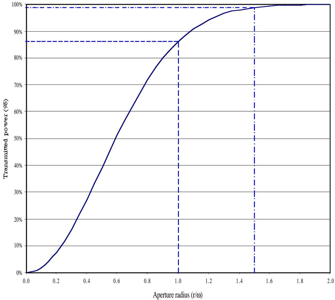
This result says that if  $a = \omega$  approximately 86% of the incident power will be transmitted through the aperture, i.e., 14% power loss. A general rule of thumb is to pick  $a \geq 1.5\omega$  at which point 99+% of the incident power will be transmitted through the aperture.
