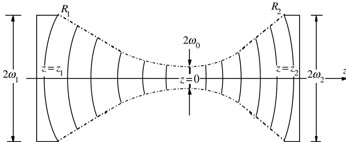
Note that as long as the mirrors are significantly larger than the spot size, the shape of the mode will depend only on  $R_1$ ,  $R_2$  and  $\ell = z_2 - z_1$  (since  $z_1 < 0$ ).
