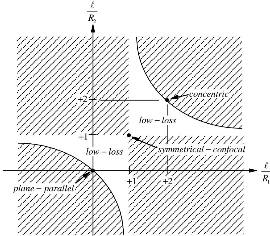
Stability diagram of an optical resonator
