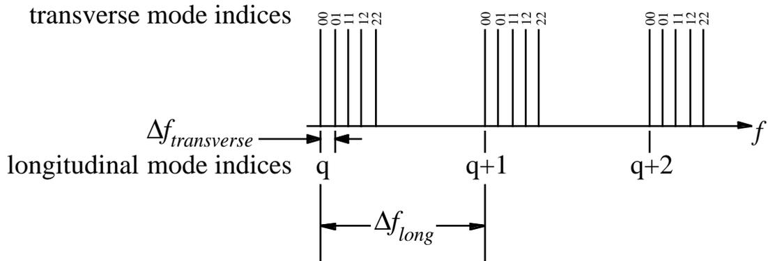
Note that the transverse mode frequencies do not continue indefinitely. Even if the laser is operating in many higher order modes simultaneously there will be a maximum transverse mode  $TEM_{mq}$  beyond which the diffraction losses become too great to allow lasing in these higher order modes.
