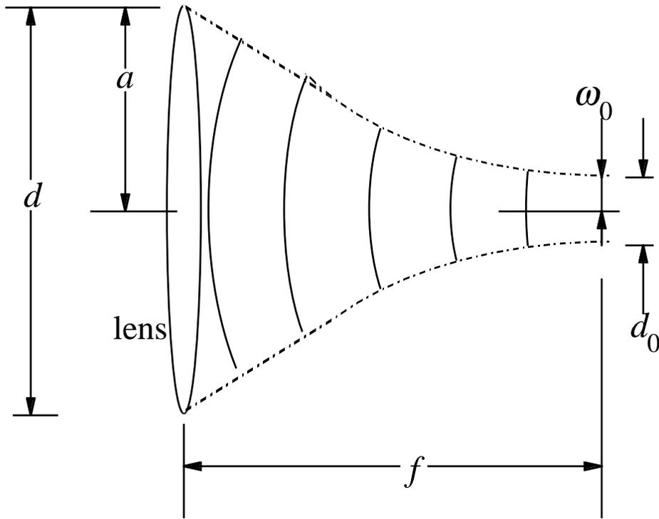
The wavefront leaving the lens is highly curved since  $f$  is generally short. This means that  $f \gg z_R$  since in the collimated beam waist the curvatures are very planar ( $R(z)$  very large).
