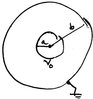
cross section of a coaxial cable.
