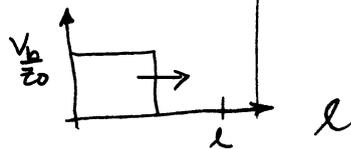
as reflection  $\Gamma = -1$  so pulse reflects inverted
