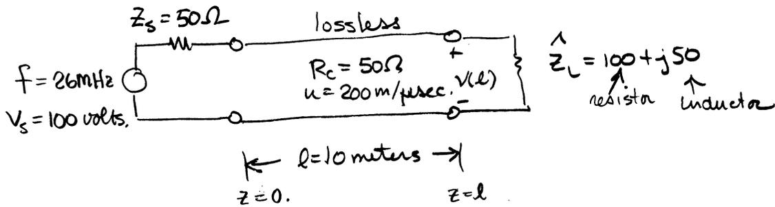
Problem: determine the input impedance to the line and the phasor voltages at  $z=0$  and  $z=l$ .
