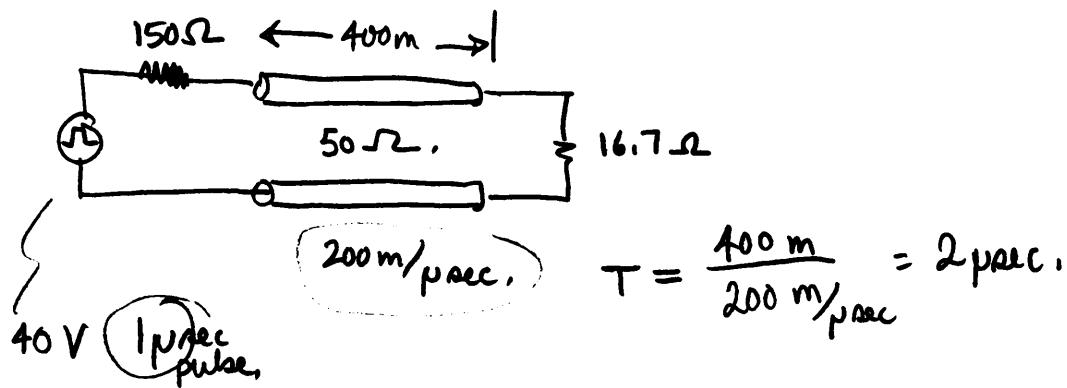
$$\text{into line: } V^+ = \frac{50}{200} (40) = 10 \text{ V.}$$
