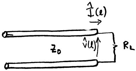
$$\text{at load } Z_L = R_L \text{ and } I(l) = \frac{\hat{V}(l)}{R_L}$$
