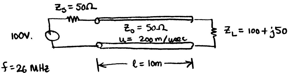
$$\beta = \frac{\omega}{u} = \frac{2\pi f}{u} = \frac{(26 \times 10^6) 2\pi}{200 \frac{\text{m}}{10^{-6}}} = 0.8168 \text{ rad/m.}$$
