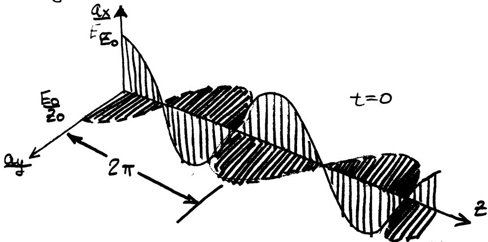
$\underline{E}$  and  $\underline{H}$  vary with a temporal frequency  $\omega$ . They also vary with a spatial frequency  $\beta = \frac{\omega}{c}$ . To illustrate, examine the above diagram for  $t=0$ . The wave repeats itself every  $2\pi$ . If we call this distance the wavelength
