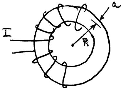
A toroid is simply a solenoid in which the ends are brought together.
