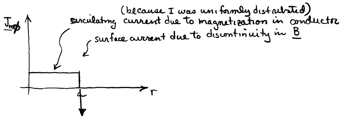
Example : Field of a permanent magnet; Find the field on the z-axis a distance  $z$  from the center of the rod of length  $L$  with magnetization  $m_s$ .
