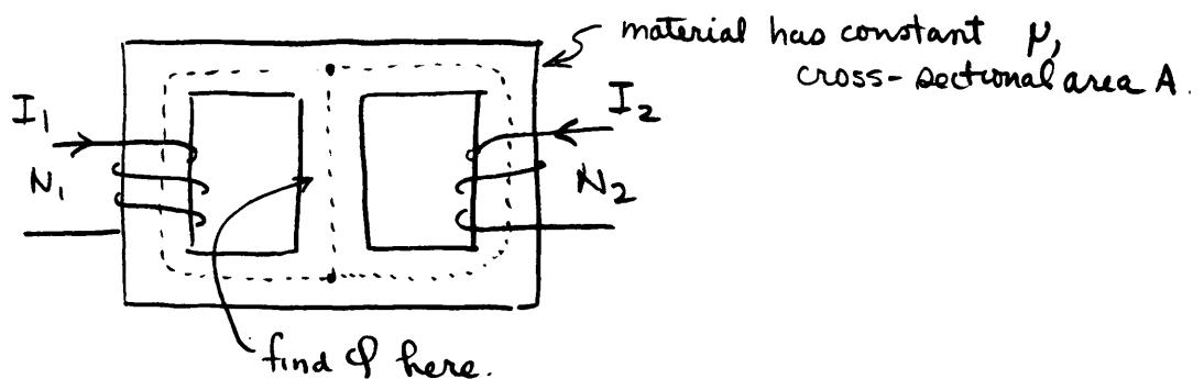
Solution : draw equivalent "electrical" circuit
