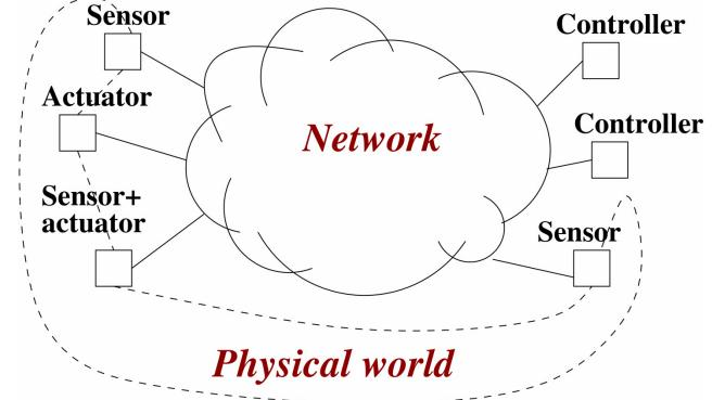
*Fig. 1.* SANETs consist of sensors, actuators, and controllers. Sensors sample the values of physical quantities and send them inside packets to controllers. Controllers examine received samples to compute control signals that are then sent to actuators. Actuators translate control signals into physical actions. All communications occur over the network [1].
