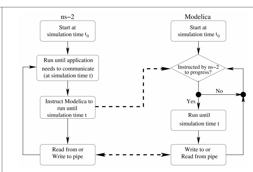
*Fig. 2.* The Modelica & ns-2 inter-simulator communication mechanics. ns-2 runs first and Modelica is paused. When the ns-2 application is slated by ns-2's event scheduler to receive (deliver) data from (to) a Modelica model at time t, it instructs Modelica to run until time t, and to exchange data at that point. After the data exchange, Modelica simulation time is suspended until the ns-2 application is scheduled again. Dashed lines represents communication via UNIX named pipes.
