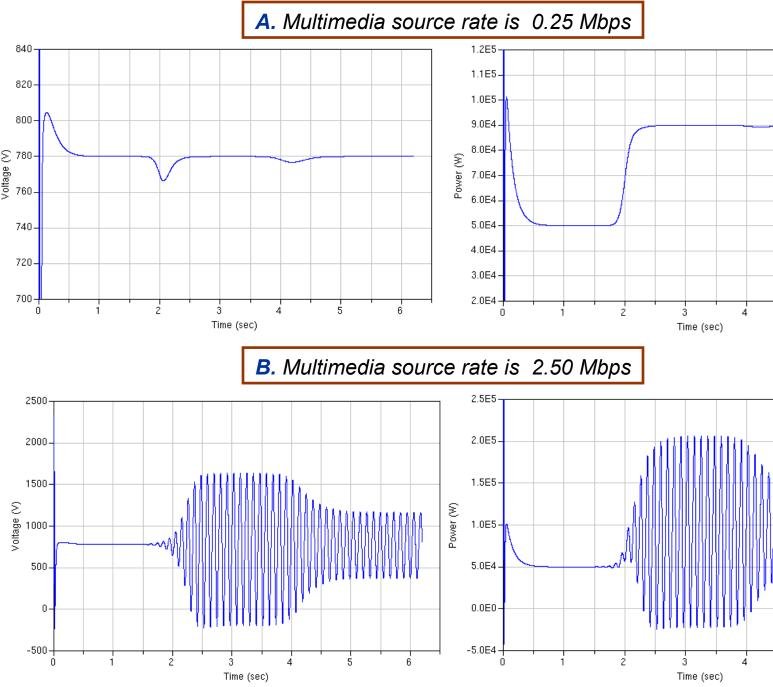
Fig. 5. The influence of the network cross-traffic on the ability of the SANET to stabilize the generator's voltage under the varying load. The plots show the line voltage and power for two cases of the multimedia transmission rate.
