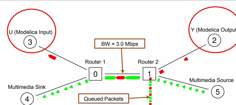
*Fig. 4.* The network topology over which voltage samples of Fig. 4 are communicated to the controller. The bottleneck link, which connects Router 1 and Router 2, has a capacity of 3.0Mbps and is shared by sensor data and multimedia cross-traffic that flows from node 5 to node 4.
