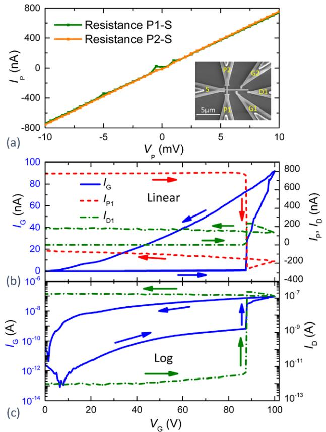
**Figure 11.** Switching behavior of a type II device (three-terminal cantilever-nanowire structure) with independent gates and drains. (a) Measured resistances from the PZR transducers P1 and P2 to S. Inset: SEM image of the device. (b), (c) Measured switching characteristics with currents measured with PZR transducer at P1 (red dashed lines) and drain current recorded at the local drain contact D1 (olive dash dot lines) in (b) linear and (c) logarithmic scales.
