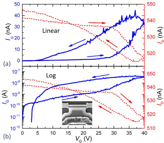
**Figure 12.** Two-terminal switching in a type III doubly clamped SiNW with  $L \approx 3.5 \mu\text{m}$ ,  $w = 320 \text{ nm}$ , and  $g \approx 200 \text{ nm}$  in (a) linear and (b) logarithmic scales. Inset in (b) shows the SEM image of the device.
