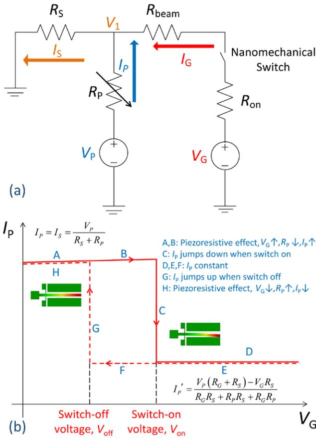
**Figure 2.** (a) Equivalent circuit model for type I two-terminal PZR SiNW switch measurement. (b) Expected behavior of  $I_P$  as  $V_G$  sweeps up (red solid line) and then sweeps back to 0V (red dashed line). Insets in (b) show the deflection profiles when the switch is off (near region A) and on (near region D).
