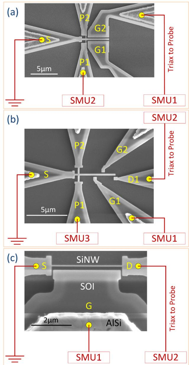
**Figure 6.** Illustration of the measurement schemes for (a) coupled cantilever-SiNW structures with two gates (G1 and G2) and two PZR transducers (P1 and P2), (b) coupled cantilever-SiNW structures with two gates, two PZR transducers, and a separate drain electrode (D1), and (c) doubly clamped SiNWs. Insets: SEM images of the devices.
