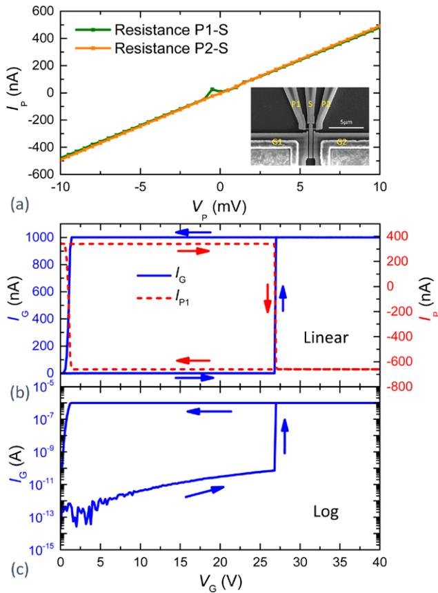
**Figure 10.** (a) Measured resistances from P1 and P2 to S of another type I device (ID: I-D). Inset: SEM image of the device. (b), (c) Measured switching characteristics of the device in (b) linear and (c) logarithmic scales.
