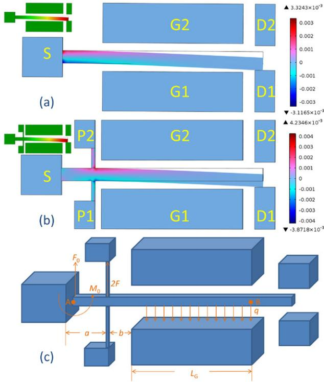
**Figure 3.** FEM simulation and mechanical analysis of type II three-terminal SiNW NEMS switch when G1 is used for actuation and the SiNW cantilever (S) is contacting drain D1. (a), (b) Strain distribution of SiNW switches (a) without and (b) with PZR transducers, where D1 and D2 are the two drain contacts. Insets in (a) and (b) show the deflection profiles. (c) Mechanical analysis of the system.
