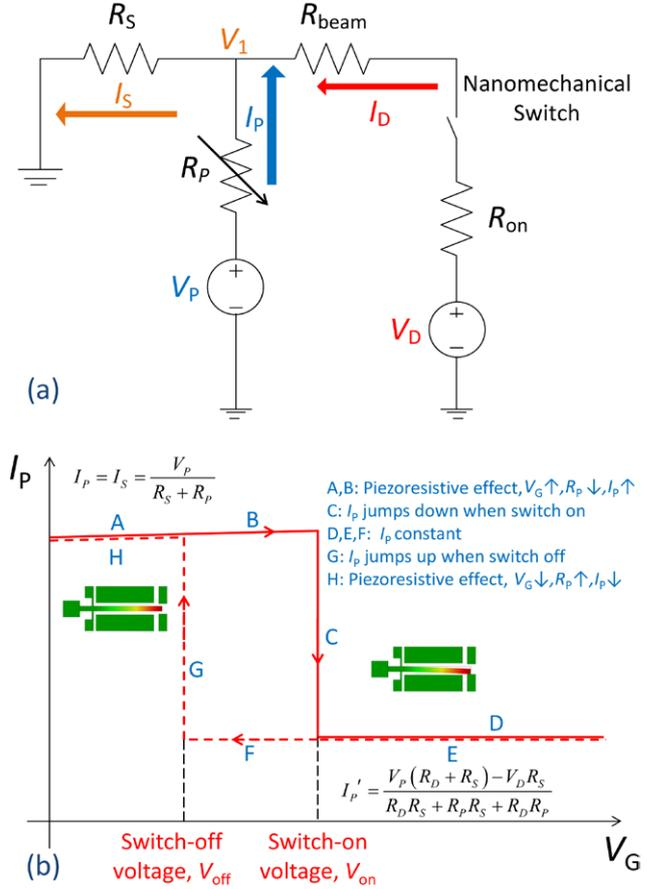
**Figure 4.** (a) Equivalent circuit model for the type II three-terminal SiNW switch PZR measurement, where  $I_D$  is the drain current. (b) Expected  $I_p$  with different  $V_G$ , where  $R_D$  is the sum of  $R_{\text{on}}$  and  $R_{\text{beam}}$ . Insets in (b) show the deflection profiles when the switch is off (near region A) and on (near region D).
